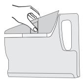
After cleaning, dry both parts of the insert thoroughly before replacing it in the water container. When replacing the insert (see illustration), guide it in at an angle ① and push the side with the opening downwards ②.
